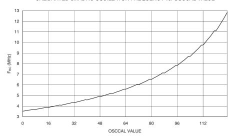
For all tunable oscillators it is important to notice that it is not recommended to tune the oscillator more than 10% off the base frequency specified in the datasheet<sup>(1)</sup>. The reason for this is that the internal timing in the device is dependent on the RC-oscillator frequency.
